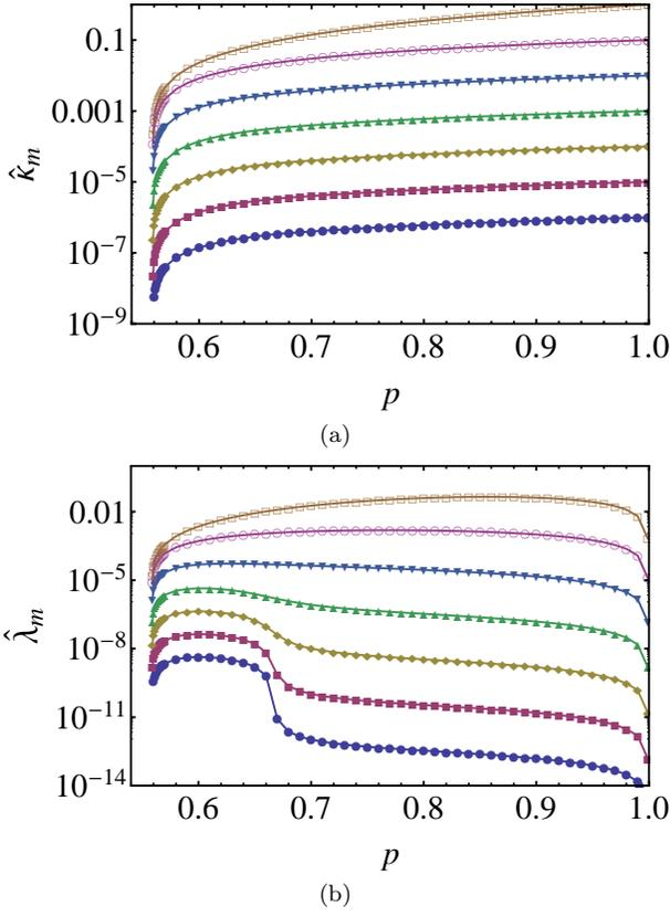
FIG. 6. (color online) The EMT solution for  $\kappa_m$  expressed in terms of the dimensionless combination  $\hat{\kappa}_m = \kappa_m/(\mu a^2)$  (a) and  $\lambda_m$  expressed in terms of the dimensionless combination  $\hat{\lambda}_m = \lambda_m/(\mu a^2)$  (b). Parameters and color code are the same as in Fig. 5.
