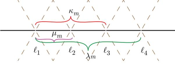
FIG. 4. (Color online) Positions of sites  $\ell_1, \ell_2, \ell_3, \ell_4$ , and interactions in the effective medium, including NN stretching term of rigidity  $\mu_m$ , NNN bending term of rigidity  $\kappa_m$ , and third neighbor effective coupling term of rigidity  $\lambda_m$ .
