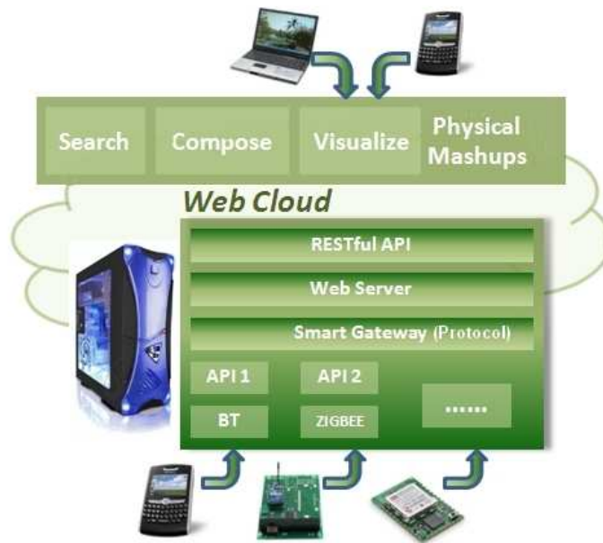
Figure 2: Smart gateway based architecture [1].
