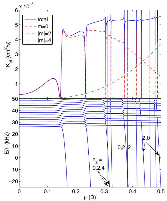
FIG. 2: Elastic collision rate as a function of  $\mu$  for a trapping frequency of  $f_z = 50$  kHz and collision energy of  $k_B \times 200$  nK, showing the contributions of the  $m = 0, \pm 2$  and  $\pm 4$  partial waves (upper panel), and the corresponding  $m = 0$  bound state calculation with  $f_z = 50$  kHz and  $f_\rho = 1$  kHz (lower panel). The  $z$  trap states with a substantial admixture are indicated for each bound state not concentrated solely in  $n_z = 0$ .
