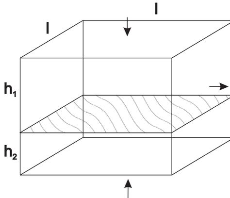
Figure 1: The system for the mechanical determination of the surface  $\Omega$ -potential of a fluid in a force field. The interface plane is singled out. The potential energies of the particles of the upper (index 1) and lower (index 2) parts are different.
