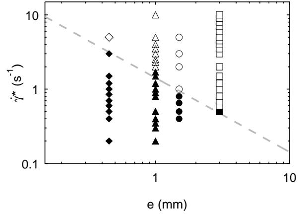
FIG. 14: Type of transient shear-banding regime as a function of the gap width  $e$  and the applied shear rate  $\dot{\gamma}$ . Filled symbols indicate a transient shear banding characterized by an induction period followed by strong fluctuations. Open symbols correspond to a fast and smooth shear-banding regime. The dashed line is  $\dot{\gamma}^* = 1.5/e$ . Experiments performed in smooth Couette geometries for different batches of 1 % w/w carbopol microgels.
