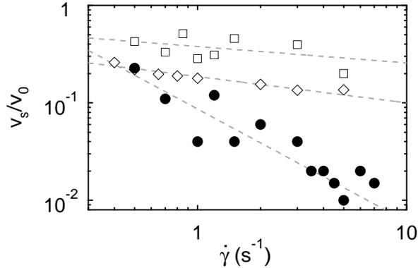
FIG. 15: Steady-state total slip velocity  $v_s$  relative to the rotor velocity  $v_0$  as a function of the applied shear rate  $\dot{\gamma}$  for smooth Couette geometries of gap width  $e = 0.45$  mm ( $\square$ ),  $e = 1.5$  mm ( $\diamond$ ), and  $e = 3$  mm ( $\bullet$ ). Dotted lines are power laws drawn to guide the eye. Experiments performed on different batches of 1 % w/w carbopol microgels.
