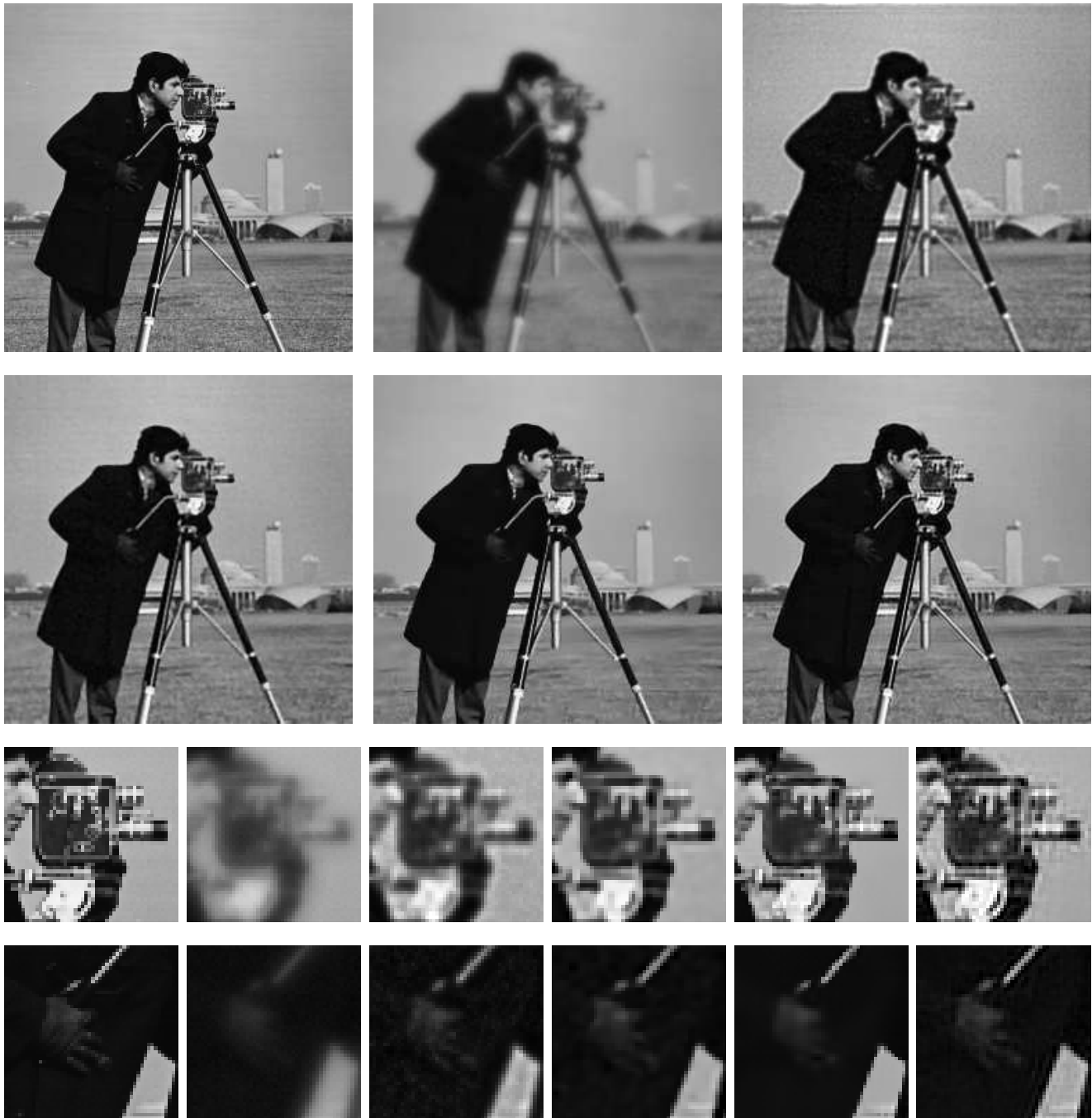
Fig. 1 Examples of deblurring and close-up for the case 2. First two lines, from top to bottom, left to right: original image, blurry image, Richardson-Lucy, sparse gradient [15], SA-DCT [10], our method. Last two lines: close-ups in the same order. Best seen by zooming on a computer screen.
