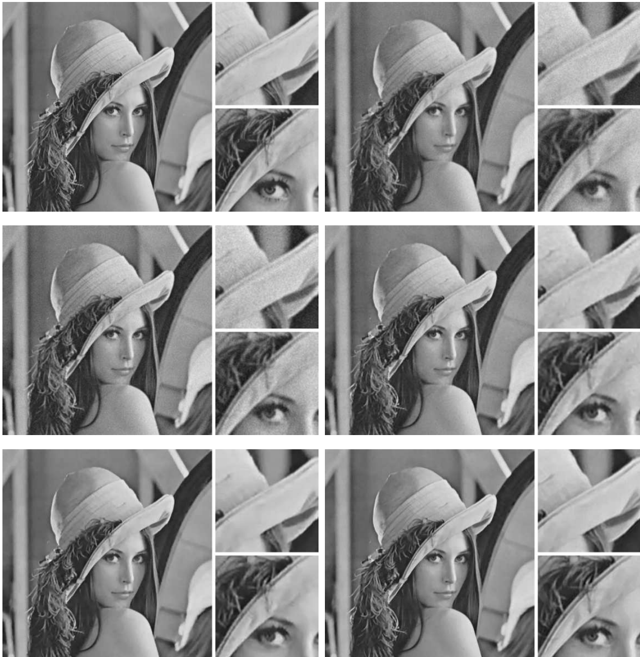
Fig. 3 Examples of deblurring for the case 4. From top to bottom, left to right: original image, blurry image, Richardson-Lucy, sparse gradient [15], SA-DCT [10], our method. Best seen by zooming on a computer screen.
