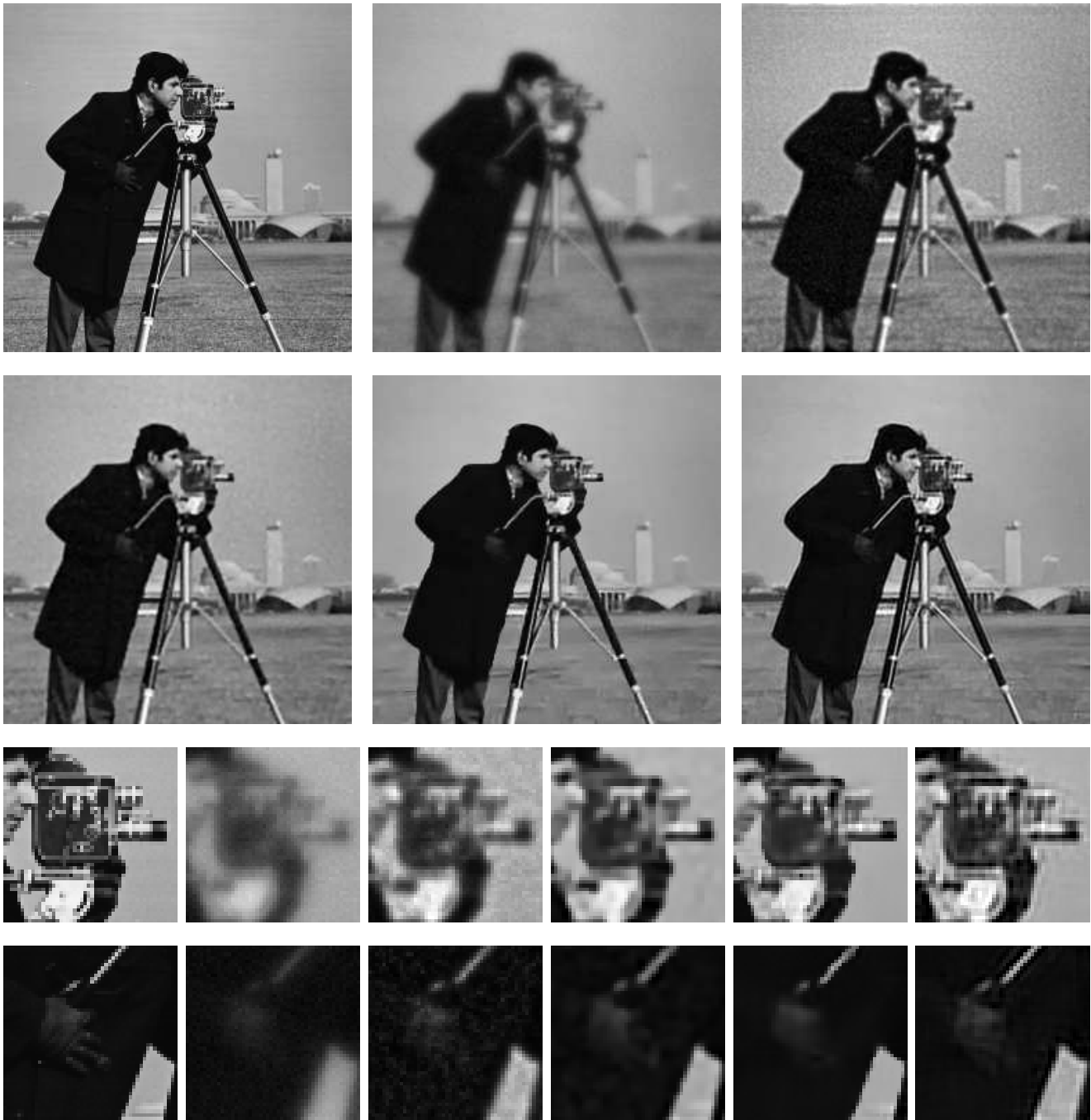
Fig. 2 Examples of deblurring for the case 3. First two line, from top to bottom, left to right: original image, blurry image, Richardson-Lucy, sparse gradient [15], SA-DCT [10], our method. Last two lines: close-ups in the same order. Best seen by zooming on a computer screen.
