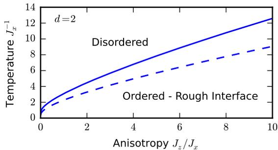
FIG. 5: (Color online) For the  $d=2$  anisotropic Ising model, the phase diagram showing the disordered phase and the ordered phase with rough interface. The dashed curve is the exact ordering boundary  $\sinh(2J_x)\sinh(2J_z) = 1$  obtained from duality. No ordered phase with smooth interface is found.
