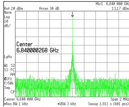
Fig 3- RF spectrum of synthesizer output
