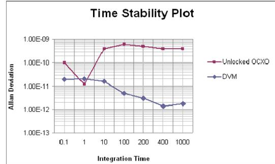
Fig 6- Allan deviation of unlocked and locked OCXO.
