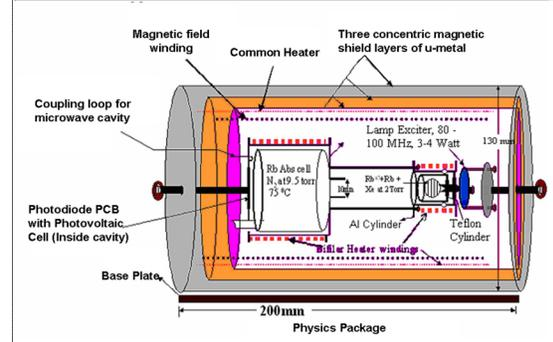
Fig.1 (b)-Detailed view of the Physics Package
