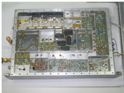
Fig 2 (b). 6.834 GHz RF Synthesizer
