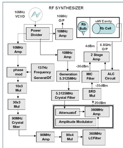
Fig 2 (a) - Schematic of 6.834GHz synthesizer.
