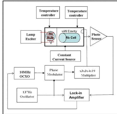
Fig.1 (a) - Functional block diagram of rubidium atomic frequency Standard
