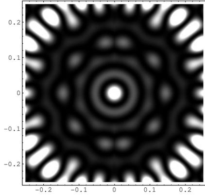
Fig. 6. Transverse intensity profile of the diffracted beam (22) by the CPSSA when the zeroth-diffraction-order beam is not eliminated. The parameters used are:  $p=9$ ,  $z=16$  cm,  $\gamma=0,0235$  rad,  $n=n'=1,48$  for incident beam wavelength  $\lambda=1$   $\mu\text{m}$ ,  $k\delta=13$ , and  $w_0=3,5$  mm.
