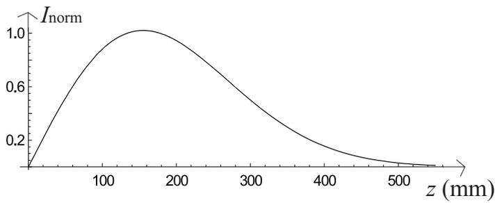
Fig. 5. Intensity variation on the bright spots situated in a circle around the central dark spot, along the beam propagation direction  $z$ , according to Eq. (23).
