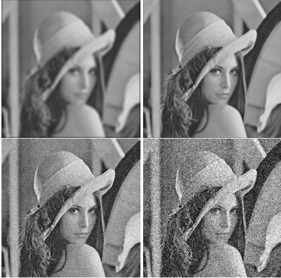
FIG. 6. Information-theoretic measures for different versions of the Lena image. From left to right and top to bottom, the results for H_\beta are: 4.6579, 4.7243, 4.9001 and 5.2040. Similarly, the results for \Phi_\beta are: 0.0580, 0.4776, 8.7643 and 17.7712. Finally, the results for \Psi_\beta are: 62.7282, 60.9517, 52.6158, 39.3270. Note that \Phi_\beta is a good measure in capturing the differences between the images.
