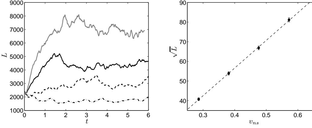
FIG. 9: Left: The evolution of the vortex line density  $L$  ( $\text{cm}^{-2}$ ) vs time  $t$  (s) for counterflow simulations at 1.9 K for four counterflow velocities: dashed-dotted,  $v_{ns} = 0.2$  cm/s, dashed,  $v_{ns} = 0.4$  cm/s, solid (black),  $v_{ns} = 0.6$  cm/s, and solid (grey),  $v_{ns} = 0.8$  cm/s. Right: The plot of the vortex line density  $L$  ( $\text{cm}^{-2}$ ) vs  $v_{ns}$  (cm/s) confirms that the saturated line density scales according to  $L \sim v_{ns}^2$ .
