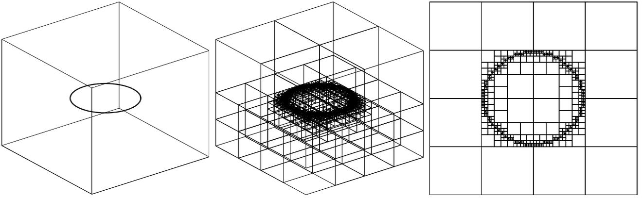
FIG. 2: The complex octree structure required to map the vortex points for a single vortex loop (left panel) is plotted in the middle panel. The right panel shows the same structure in the  $xy$ -plane, at  $z = 0$ .
