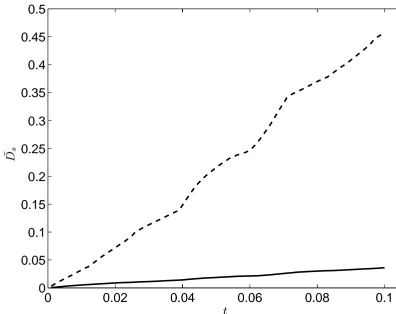
FIG. 8: The evolution of the normalised distance error statistic  $\bar{D}_s$  (see Eq. (27)), for a system of leap-frogging vortex rings, plotted as a function of  $t$  (seconds). The solid line corresponds to a simulation with  $\theta_{\max} = 0.4$ , and the dashed line to  $\theta_{\max} = 0.8$ .
