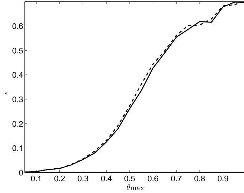
FIG. 5: The scaling of the mean relative percentage error in the velocity field,  $\bar{\epsilon}$ , evaluated at discretization points plotted as a function of  $\theta_{\max}$ . The dashed line corresponds to the original opening angle criterion [49] and the solid line shows the performance of the correction of Barnes [55].
