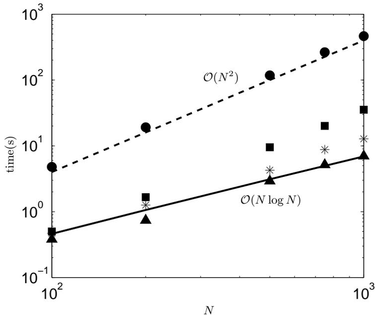
FIG. 4: The CPU time required for one hundred time-steps, plotted as a function of the number of vortex points  $N$ . The calculations were performed on a single processor with a clock speed of 2.53 GHz. The symbols represent different values of  $\theta_{\max}$  as follows: triangles,  $\theta_{\max} = 0.6$ , asterisks,  $\theta_{\max} = 0.4$ , squares,  $\theta_{\max} = 0.2$ , and circles,  $\theta_{\max} = 0$ . (that is, the full BS calculation).
