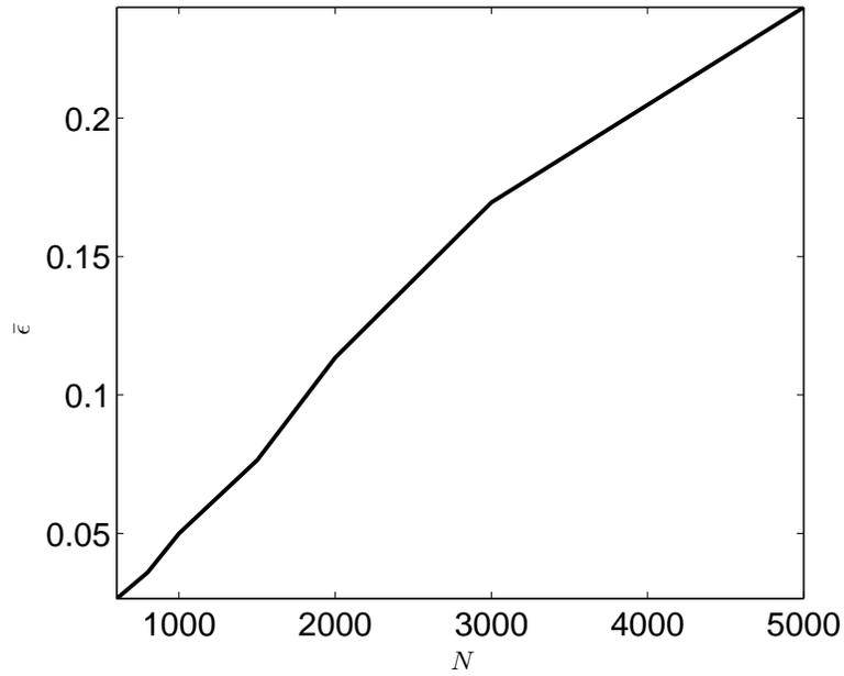
FIG. 6: The mean relative percentage error of the tree approximation for a fixed maximum opening angle,  $\theta_{\max} = 0.4$ , with an increasing number of discretization points and therefore vortex length in the system.
