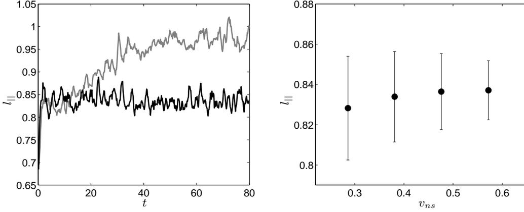
FIG. 10: Left: The anisotropy parameter  $l_{\parallel}$  plotted as a function of time  $t$  (s) for the LIA simulation (grey) and for the tree method (black) with  $\theta_{\max} = 0.4$ . Right: The steady-state  $l_{\parallel}$  parameter plotted for four different normal fluid velocities  $v_{ns}$  (cm/s) plotted with error bars (calculated from temporal fluctuations) for the tree method only. These results are in excellent agreement with those of Adachi *et al.* [45]
