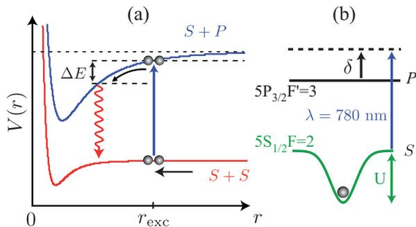
FIGURE 1: (a) Light-assisted atom loss by radiative escape. Atoms in the  $S$  state interact through the Van der Waals potential  $V(r) = -C_6/r^6$  while atoms in the  $S$  and  $P$  states interact through the dipole-dipole attractive potential  $V(r) = -C_3/r^3$ . (b) Levels involved in the experiment. The excitation laser detuning  $\delta$  is measured with respect to the free space transition.
