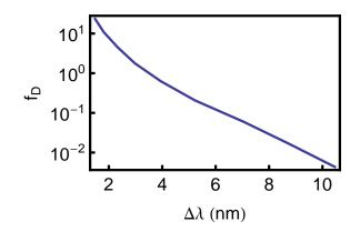
Fig. 5. (Color online) Theoretically-predicted best achievable fractional delay vs. input pulse bandwidth (centered at  $\lambda_c$ ) subject to the constraint that  $D_a, D_p < 0.05$ , which corresponds to negligible distortion (*i.e.*, just noticeable upon visual inspection).
