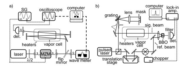
Fig. 1. Schematics of the experimental setups. a) A weak beam is modulated by a MZM, passes three times through a heated Rubidium vapor cell (Triad Technologies, TT-RB-75-V-Q-CW), and is detected by a fast photoreceiver (New Focus 3051). b) An ultrashort pulse passes once through the vapor cell, overlaps with a tunable reference pulse in a BBO crystal, and the resulting sum-frequency generated light is recorded.
