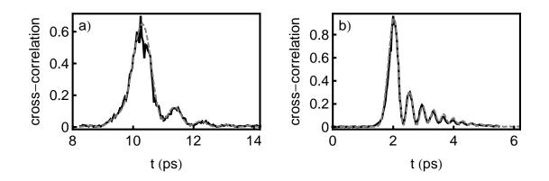
Fig. 3. (Color online) Comparison of experimental (solid line) and theoretically predicted (dashed line) results for a a) 650-fs-long pulse centered at  $\lambda_c$  and a vapor temperature of 326 °C and b) 250-fs-long pulse centered at 787.5 nm and a vapor temperature of 263 °C.
