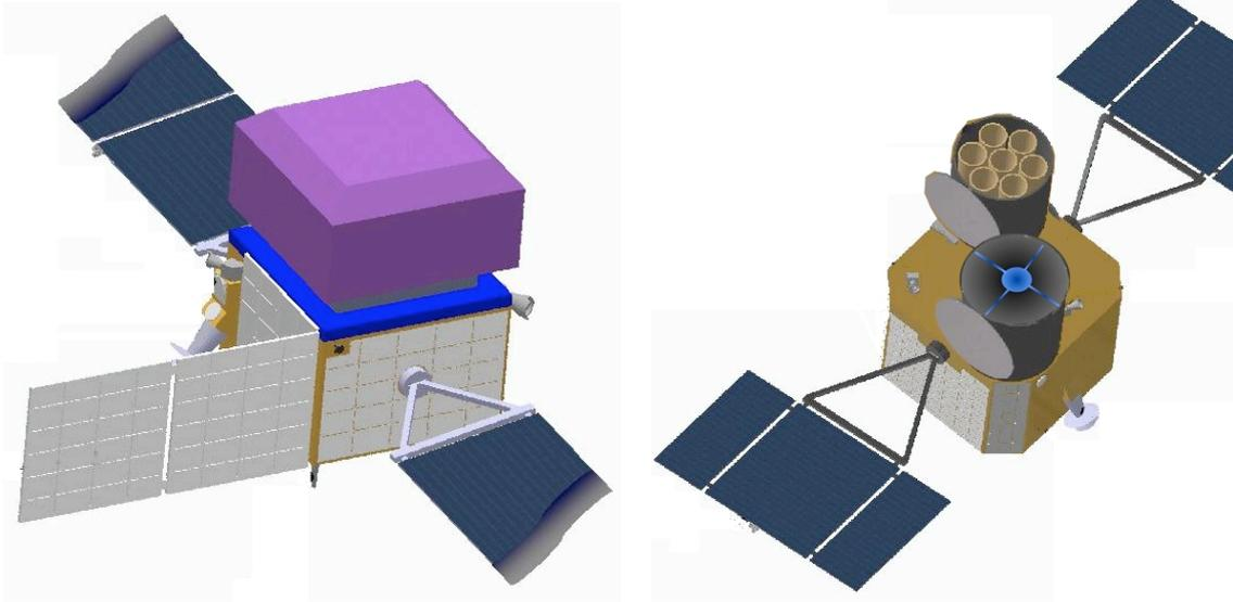
**Figure 2:** GRIPS configuration in the two-satellite option, where the GRM is on one satellite (left), and XRM and IRT on the other (right). The GRM satellite would just do the zenith scanning all-sky survey, while XRM/IRT would re-point with the whole (second) satellite to GRBs, similar to *Swift*.
