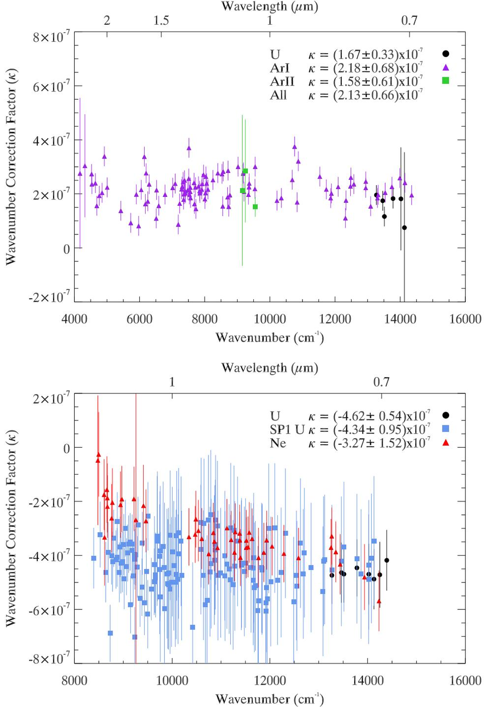
Fig. 2.— **Top:** Wavenumber correction factor of SP1, using wavenumber standards from Whaling et al. (2002); Sansonetti (2007) (ArI and ArII lines) and Degraffenreid & Sansonetti (2002) (U lines). Uncertainties in this plot are calculated via Equation 3. **Bottom:** The same, but for SP3 (U/Ne). The neon standards come from Sansonetti et al. (2004), and a comparison to the uranium lines of SP1 are from this work.
