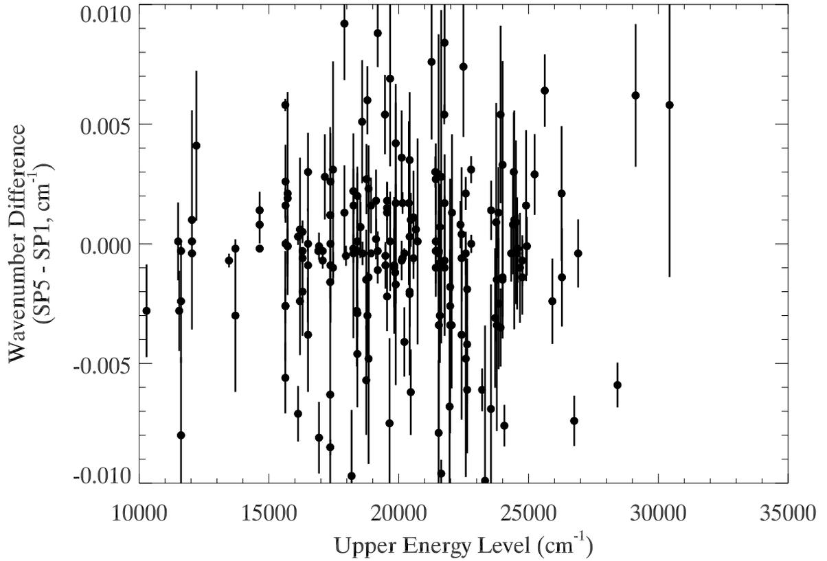
Fig. 4.— The wavenumber difference (in  $\text{cm}^{-1}$ ) between our highest-current spectrum (SP5, 300 mA) and our lowest-current spectrum (SP1, 26 mA) as a function of the upper energy level of the transition. The uncertainties are the sum in quadrature of the uncertainties in SP1 and SP5. The lack of a trend indicates that plasma shifts are not an issue for these upper energy levels.
