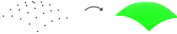
FIG. 4: (Color online) Construction of a locally smooth parameterization starting from a point cloud.
