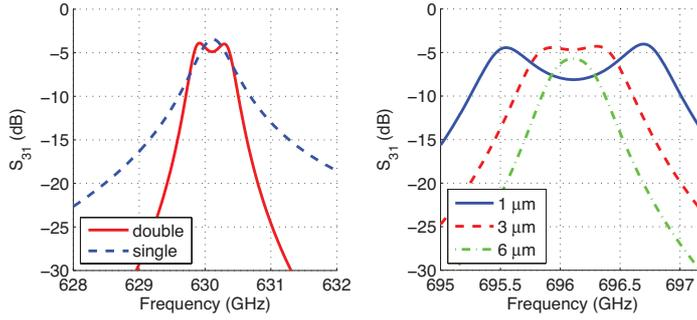
**Fig. 3** (Color online) a) Calculated transmission  $S_{31}$  of filters with 1 (dashed) and 2 (solid) halfwave resonators. The geometry of the simulated model is described in Fig. 2, with  $G = 3 \mu\text{m}$  and  $L_c = 15 \mu\text{m}$ .  $L_{\text{res}}$  has been adjusted so that the center frequency is equal in both cases. b) Transmission  $S_{31}$  of a filter with 2 coupled resonators with varying gap width  $G$ .
