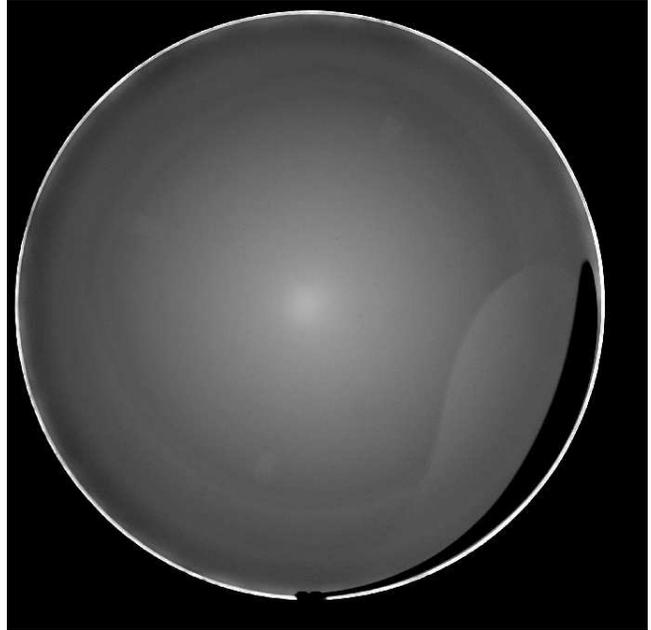
FIG. 7.— Flat field frame obtained with DomeLight in the V-band. The effect of the solar shutter is shown in the image. This effect also appears in the sky frames but it is corrected by the flat fields.
