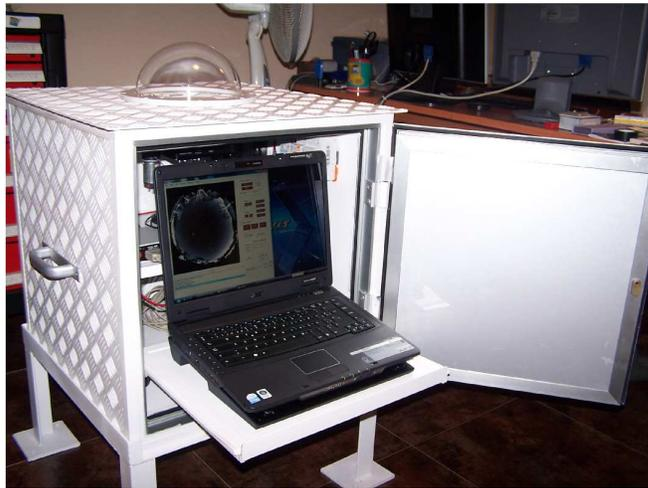
FIG. 1.— The figure shows an external view of an ASTMON unit. The internal components are protected by a weather - proof housing, so the instrument can be installed out-doors.
