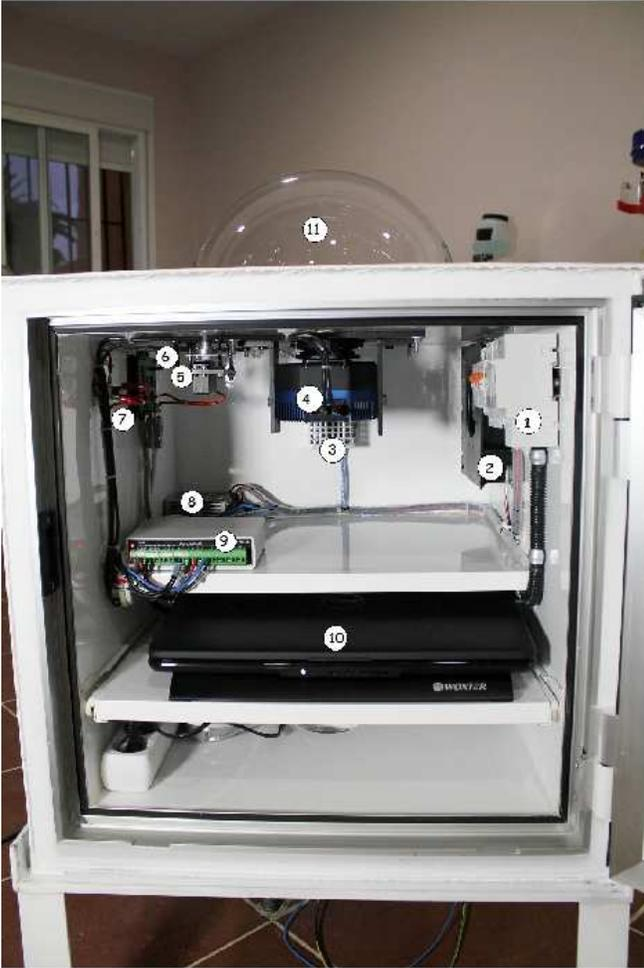
FIG. 2.— The figure shows the internal view of the system: (1) Ground fault and electrical breakers. (2) Main fan. (3) Anti-humidity system. (4) CCD head with filter wheel. (5) Servo-motor of the solar shutter. (6) Servomotor controller. (7) Thermostats. (8) Main stabilized power supply. (9) PIC I/O controller. (10) Computer. (11) Acrylic dome.
