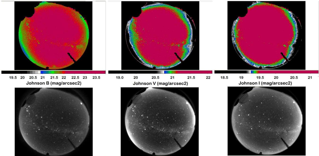
FIG. 11.— The final result of ASTMON is to provide a completely processed sky brightness map sequence of the whole sky for all the available filters as it is shown in this figure. Upper panel: Processed sequence. Each color represents different skybrightness level. Lower panel: Raw images. Data obtained by ASTMON at the Calar Alto observatory during July of 2010.
