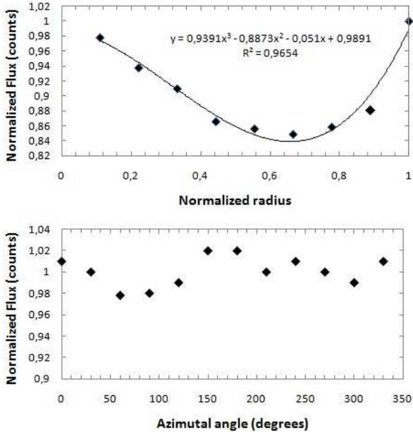
FIG. 6.— Estimation of the illumination correction of the DomeLight device. The top panel shows the radial distribution of the intensity measured with the two apertures sensor, and the bottom panel shows the azimuthal one. In both cases the intensity is normalized to the intensity at the zenith. The solid line in the left panel shows the best fitted 2nd order polynomial function.
