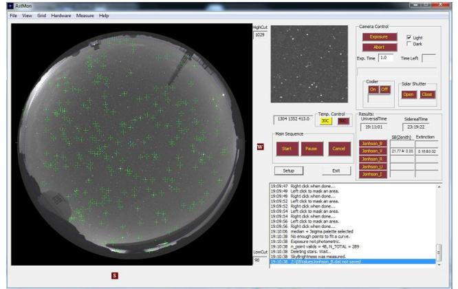
FIG. 3.— Snap-shot of the custom software developed for ASTMON, taken during one of the calibration runs. Different control buttons, entries, and panels showing the status of the instrument are seen at the right-side of the program. The panel at the left side shows one particular image of the night-sky. The green circles indicate the location of the detected stars that match with the corresponding ones at the astrometric/photometric catalogue, as described in the text.
