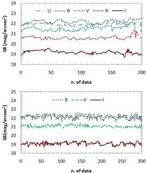
FIG. 10.— Monitoring of the night-sky surface brightness at the zenith for a complete month. Upper panel: data obtained at the Calar Alto observatory during January of 2011. Lower panel: data obtained at the Doñana National Park during May of 2010.
