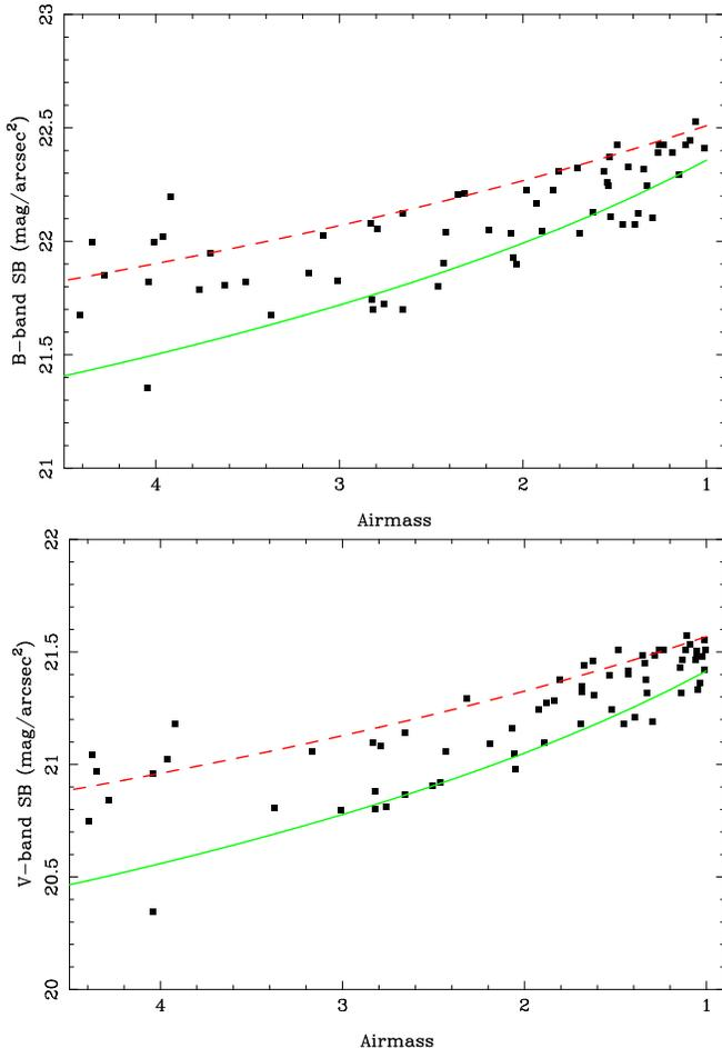
FIG. 9.— Distribution of the night sky surface brightness versus airmass for two of the five filters installed in the instrument: the B-band (top panel) and the V-band (bottom panel). The red dashed-line shows the expected distribution in the absence of light pollution, while the green solid-line shows the distribution when a  $\sim 15\%$  of light pollution is taken into account.
