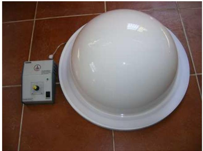
FIG. 5.— Picture of DomeLight. This device has been developed to shine uniformly any wide-field camera.
