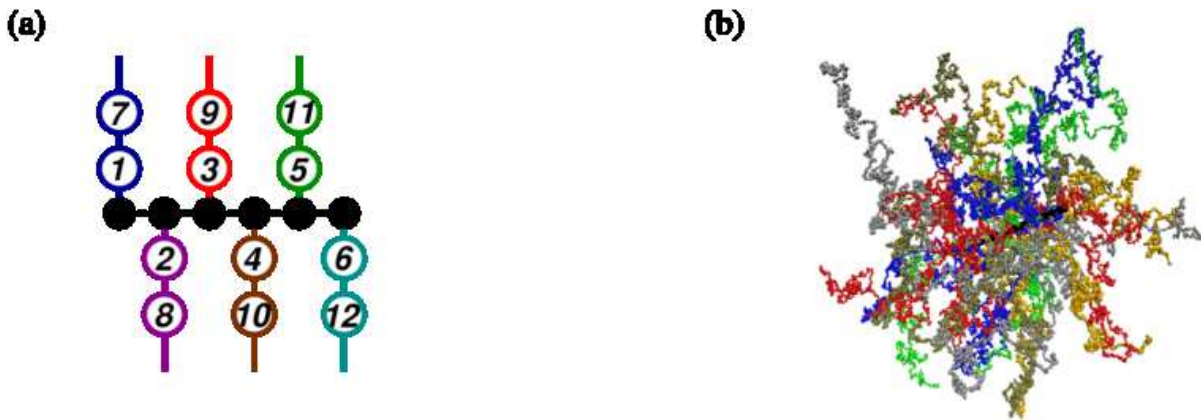
FIG. 13. (a) A schematic drawing of growing a bottle-brush polymer step by step. (b) A snapshot of the configurations of bottle-brush polymers consisting of N_b = 128 backbone monomers, N = 2000 monomers in each side chain, and the grafting density \sigma = 1/4 under a very good solvent condition generated by PERM.
