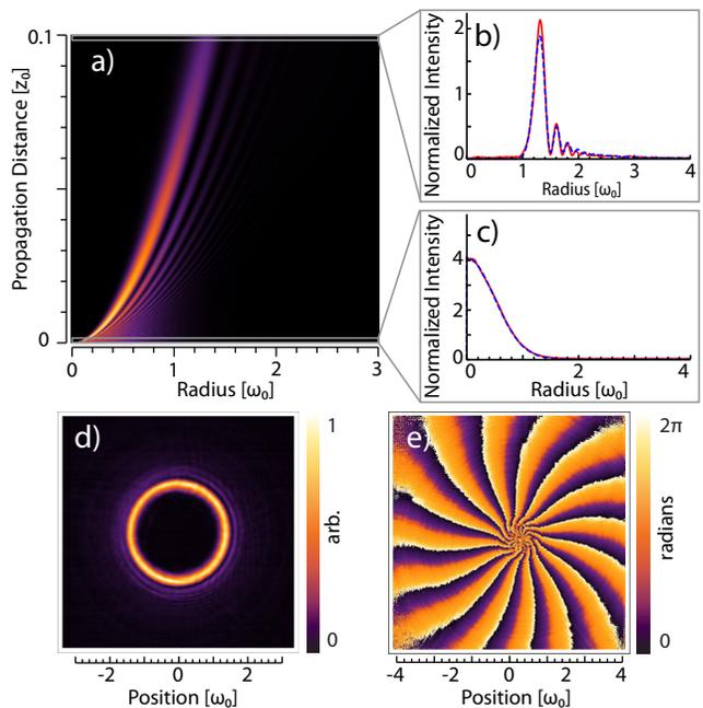
FIG. 2. a) Calculated intensity of the mode produced by illuminating a charge 15 spiral phase mirror with a collimated  $TEM_{00}$ . b), c) Measured (solid red trace) and calculated (dashed blue trace) radial intensity profiles after propagation and at the location of the SPM, respectively. d) Measured intensity profile for a charge 15 optical vortex imaged in the far-field. e) Measured phase of the same vortex imaged in the near-field.
