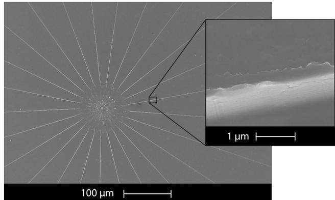
FIG. 1. Scanning electron microscope image of the central region of a charge 100 spiral phase mirror. The inset shows the edge of one of the steps.
