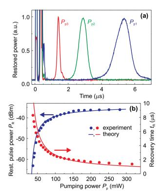
FIG. 2. (Color online) (a) The normalized time profiles of the restored signal measured at field H = 1860 Oe for different pumping powers:  $P_{\rm p1} = 50$  mW,  $P_{\rm p2} = 90$  mW,  $P_{\rm p3} = 320$  mW. (b) Measured and calculated dependencies of the restored signal power and recovery time as a function of the pumping power.
