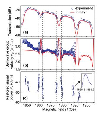
FIG. 4. (Color online) (a) Transmission of the spin-wave signal as a function of bias magnetic field (open circles - experiment, line - theory). (b) Dependence of the group velocity  $v_{\rm gr}$  on the field H. The slight decrease in  $v_{\rm gr}$  at the edges of the band gap is visible. (c) Measured restored signal power  $P_{\rm R}$  as a function of field H. One sees that the restored signal is visible only at the edges of the band gaps.
