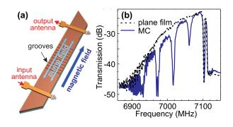
FIG. 1. (Color online) (a) Sketch of the experimental setup. The MC is fabricated in the form of YIG spin-wave waveguide with 10 grooves on its surface. The Rf pump magnetic field is parallel to the bias field H. (b) Measured transmission characteristics (the ratio of the output signal intensity to the input) of the plane YIG film and MC for the magnetic field H = 1800 Oe. Several band gaps are seen.
