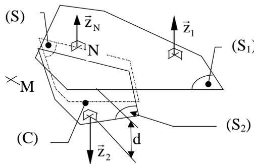
**Figure 3: Contact specification between two nominal parallel planes.**
