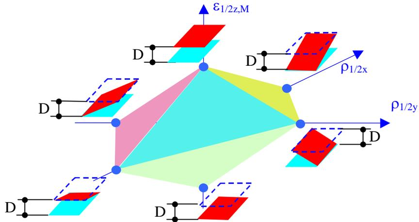
**Figure 7:** 3-polytope in  $R^3$  from contact specification between two rectangular planes.
