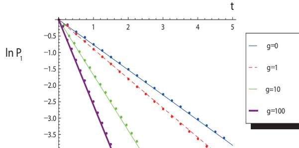
FIG. 3:  $\ln P_1(t)$  plots for various  $g$  (different colors). Dots are from numerical simulation and lines are from theoretical prediction of decay rate by outgoing boundary conditions of (41) and (42). The numerical simulation and theoretical prediction show very good agreement.
