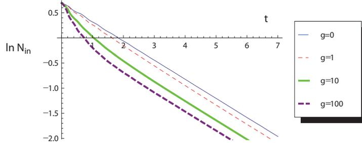
FIG. 9:  $\ln N_{\text{in}}(t)$  plots. For smaller  $g$  it is closer to the straight line (exponential decay) but for larger  $g$  the decay rate changes from faster to slower ones.
