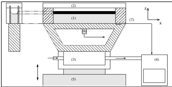
FIG. 1: Schematic of the set up. A parallelepipedic cell (1) sealed by a plexiglass lid (2) and thermostated by water circulation (3) from a thermostated bath (4) is vertically vibrated by an electromagnetic shaker (5). The amplitude of the oscillation is recorded via an accelerometer (6), while the temperature of the cell is measured with a probe (7) and feedbacked to the water bath. Left: side view of the cell.
