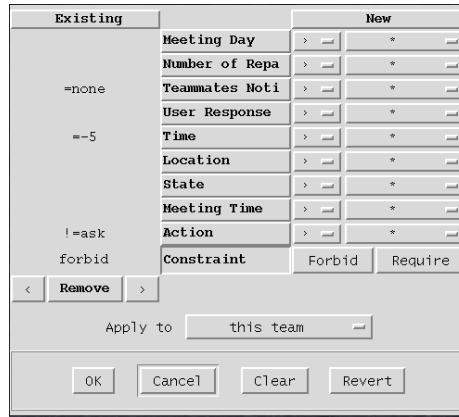
Figure 6: Screenshot of the tool for entering constraints. The constraint displayed forbids not transferring control (i.e., forces transfer) five minutes before the meeting if the teammates have previously been given information about the user’s attendance at the meeting.
