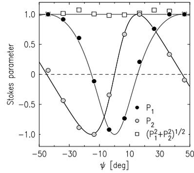
**Fig. 5.** Left: Measurement of the Poincaré-Stokes parameters as function of the azimuthal angle at the Ge (006) reflection. Solid lines are fits to eq. 41. Right: Poincaré-Stokes parameters extracted from the measurements shown on the left by fitting to eq. 41. The experimental values are in quite satisfactory agreement with the parameter-free predictions (eqs. 42 and 43), show as lines. Taken from [32].
