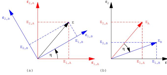
**Fig. 3.** A change of the coordinate system from  $A$  to  $B$  is effected by an orthogonal rotation matrix. (a) Transformation of the coordinate system relative to a fixed laboratory reference. (b) Transformation of the vector components in these coordinate systems.
