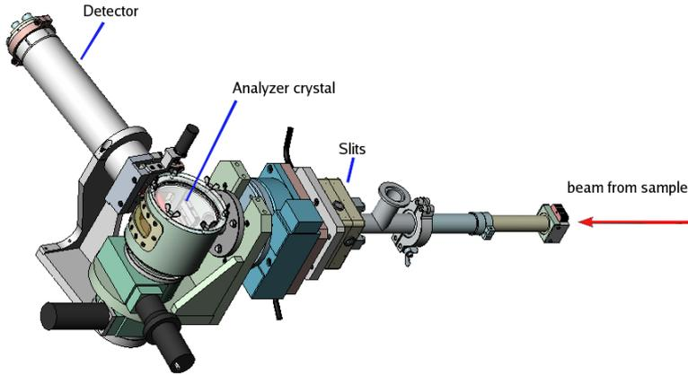
**Fig. 4.** Experimental configuration for linear polarization analysis of X-rays at the ESRF Beamline ID20 [25]. The beam scattered off the sample enters an evacuated flight tube (right). In-vacuum slits are positioned upstream of the analyzer crystal. The analyzer crystal and detector are mounted on a common goniometer rotating about the beam ( $\eta$ -axis). The Bragg ( $\theta_{PA}$ ) and scattering angles ( $2\theta_{PA}$ ) can be adjusted individually.
