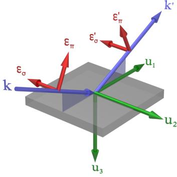
**Fig. 2.** Coordinate system and polarization vectors relative to the incident ( $\mathbf{k}$ ) and scattered ( $\mathbf{k}'$ ) beams.
