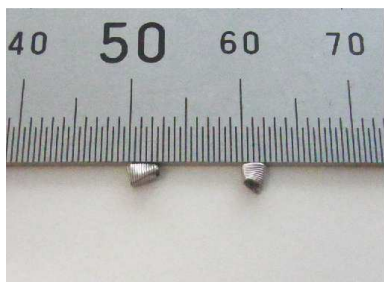
Figure 4: Photograph of Heli-packs which are filled into the rectification and reboiler parts.
