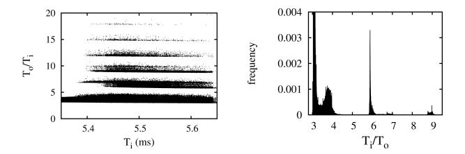
FIG. 9: Left: The ratio of the output period  $T_o$  to the input period  $T_i$  between the 3:1 and 4:1 entrained states for a biphasic pulse at  $I_0 = 45.8 \mu \text{A/cm}^2$ . Right: Histogram of response modes at  $T_i = 5.55 \text{ms}$  and  $I_0 = 45.8 \mu \text{A/cm}^2$ . The calculations were carried out for stimulus with no inter-phase gap,  $\tau = \tau_1 = 0.6 \text{ms}$ . The histogram bin size is 0.01ms. Note the absence of modes 5.8,11,14, and 17.
