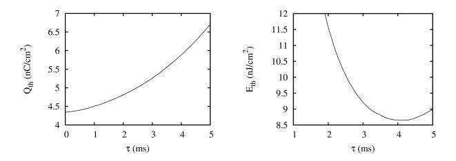
FIG. 17: Threshold charge (left panel) and threshold energy (right panel) as a function of  $\tau$  for a resonant stimulation,  $T_i = 17 \text{ms}$ , by a biphasic periodic sequence of pulses with an optimal interphase gap,  $\tau_1 = 5 \text{ms}$ . The minimum charge occurs at  $\tau \to 0$  which means that the most effective pulses are those with the shortest possible width. The pulse energy has a minimum near  $\tau = 4 \text{ms}$ .
