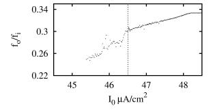
FIG. 8: The firing rate as a function of the stimulus amplitude for  $T_i = 5.5$ ms and no delay between the phases of the pulse,  $\tau = \tau_1 = 0.6$ ms. The vertical broken line separates bistable and monostable regions.
