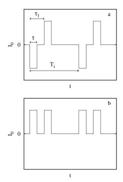
FIG. 1: Stimulus waveform used in the calculations: (a) charge-balanced biphasic form with delay, and (b) monophasic pulses with delay. The delay between the onset of the cathodic and anodic phase is  $\tau_1$  and  $\tau$  is the width of each phase.
