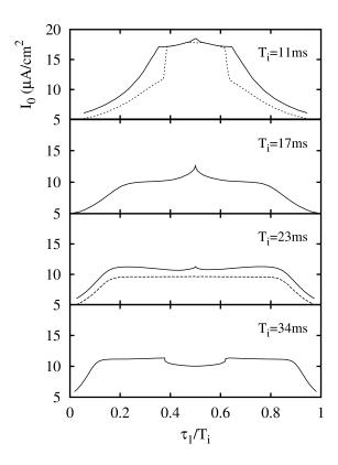
FIG. 16: Excitation edge for a double pulse as a function of separation between the leading and the trailing phase. The inter-phase gap is scaled in units of the stimulation period  $T_i$ . The diagrams from top to bottom are drawn for  $T_i = 11, 17, 23$ , and 34ms, respectively.
