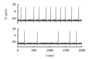
FIG. 15: Sample V(t) dependence near the resonance at  $T_i=18.2 \mathrm{ms}$ , for stimulation by biphasic pulses with  $\tau=0.6 \mathrm{ms}$ ,  $\tau_1=5 \mathrm{ms}$ . The current amplitude in the top and bottom panel is  $I_0=7.33 \mu \mathrm{A/cm}^2$ , and  $7.303 \mu \mathrm{A/cm}^2$ , respectively.
