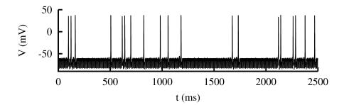
FIG. 5: Sample V(t) run for  $T_i = 8.35$ ms, very close to the multimodal transition. Here  $\tau = \tau_1 = 0.6$ ms, and the stimulus amplitude is  $I_0 = 35\mu\text{A/cm}^2$ . The shown ISI sequence is  $3, 5, 41, 13, 3, 7, 15, 19, 9, 15, 59, 7, 46, 3, 14, 3, 11, 11, in units of <math>T_i$ . The ISIs are mostly odd multiples of  $T_i$ .
