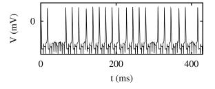
FIG. 10: Sample V(t) dependence for  $T_i = 5.55$ ms. Here  $\tau = \tau_1 = 0.6$ ms, and the stimulus amplitude  $I_0 = 45.8 \mu \text{A/cm}^2$  is slightly above threshold. The modes 3:1 and 4:1 dominate, with no clear separation between them. The modes (5+3n):1, where  $n=0,1,2,\ldots$ , do not appear in the neuron's response.
