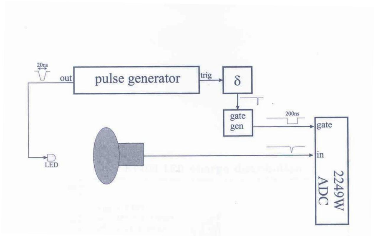
Figure 6: The test setup scheme.
