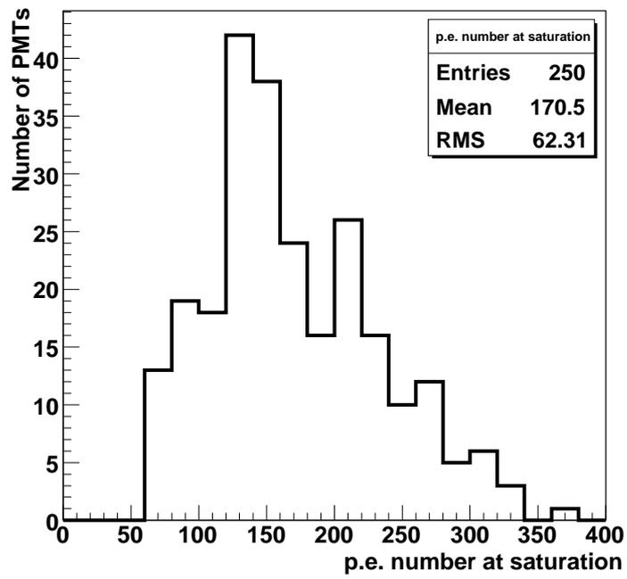
Figure 8: The PMTs saturation level obtained with the photo-statistics method(using the original linear bases).
