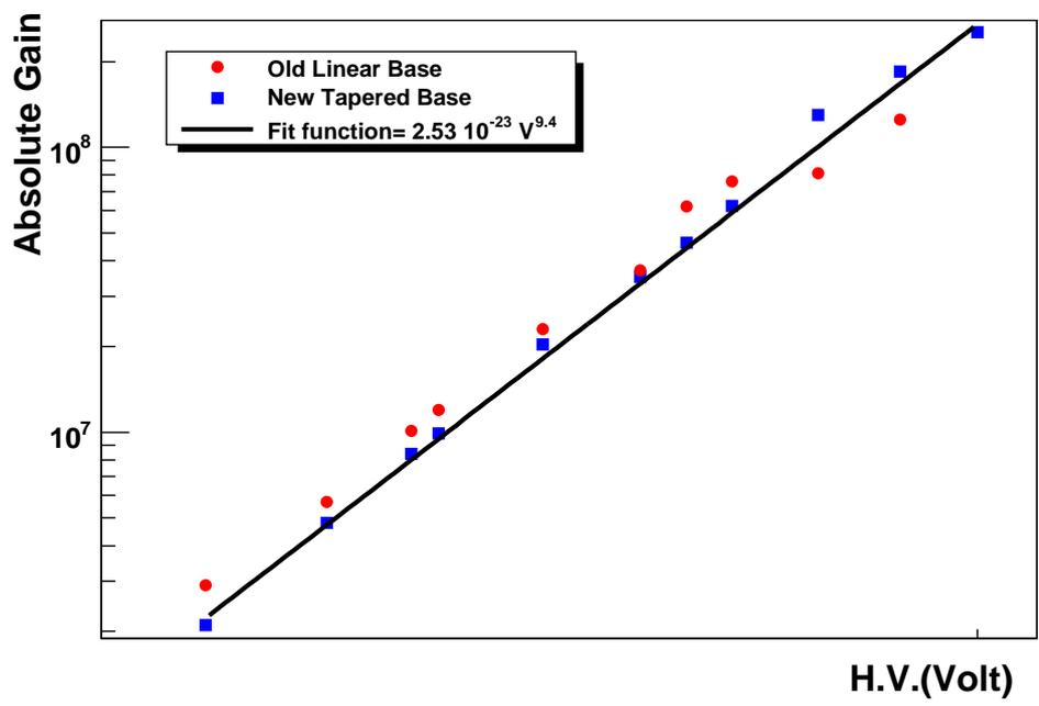
Figure 17: The absolute gain, for the PMT 1, as function as of the high voltage, the fit is for the data obtained with the tapered base.
