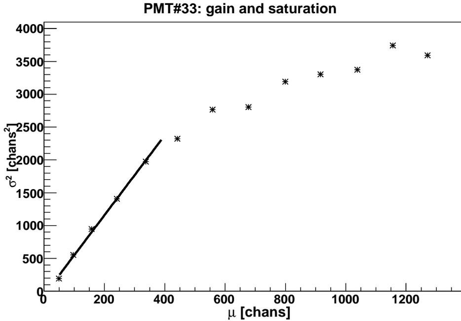
Figure 2: ADC variance( $\sigma^2$ ) versus ADC mean( $\mu$ ) for a variety pulse heights. The slope of the fit of the linear region gives the gain, and the *saturation level* =  $441/3.04 = 145$  photo – electrons.
