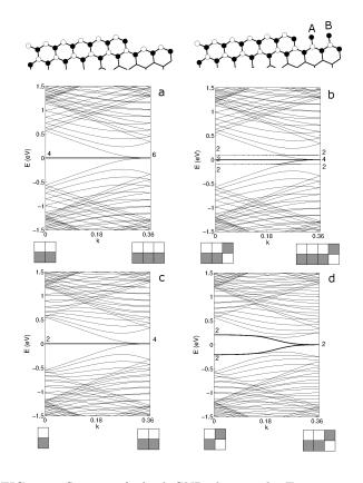
FIG. 10. Spectra of 3(8,1) GNR close to the Fermi energy with different edge terminations, ranging from the minimal edge (a) to the modified edge with one Klein node, marked as A, added (b-c) or two Klein nodes A and B attached (d). In (b)  $t = 0.1t_0$ , while in (c) and (d)  $t = t_0$ . The top panels show the minimal and modified edges.
