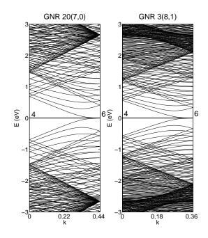
FIG. 4. Energy spectra of the 20(7,0) GNR (left) and the 3(8,1) GNR (right) close to the Fermi energy. The unit cells of both GNRs contain similar number of nodes. The degeneracies of the zero-energy edge bands (4 and 6) are indicated close to extreme k values.
