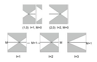
FIG. 2. Schematic band structures of zigzag (1,0), (2,0) and general (S,0) edges after folding the (1,0) zigzag edge band, where S = I + 3M as described in the text. The shaded areas represent the band continuum of states. Degeneracies of the zero-energy bands (M, M+1) are indicated in the lower panels close to the corresponding edge bands at the Fermi energy. They correspond to semi-infinite graphene sheet with only one edge. In case of a GNR with equal edges the degeneracies are doubled.
