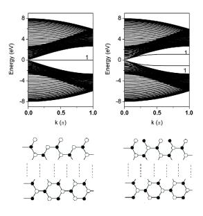
FIG. 9. Spectra of armchair GNRs with Klein nodes added to the edge. Left: 40(1,1) armchair GNR with one Klein node per unit cell. Right: the same GNR but with two Klein nodes per unit cell.
