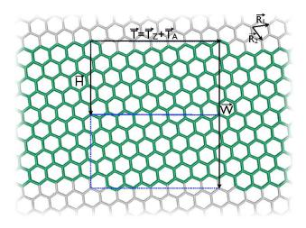
FIG. 3. (*Color online*) Geometric structure of the 2(7,1) GNR highlighted in dark grey (green) on a graphene sheet, indicating the translation vector  $\mathbf{T} = \mathbf{T}_Z + \mathbf{T}_A$  and the width vector  $\mathbf{W} = 2\mathbf{H}$ , where  $\mathbf{H}$  is the smallest nanoribbon width vector belonging to the graphene lattice.  $\mathbf{T}_Z = 6\mathbf{T}(1,0)$ . The unit cells spanned by  $\mathbf{T}$  and  $\mathbf{H}$  or  $\mathbf{W}$  are marked.
