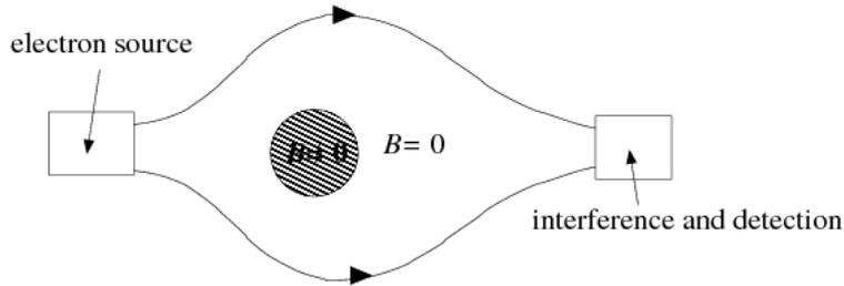
Figure 1.5: Schematic diagram of the experimental set up required to view the AB effect. The magnetic field is confined to a region from which the electrons are excluded.
