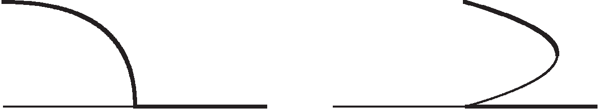
Figure 1: Schematic Diagrams of the Forward and Backward Bifurcations. The horizontal direction is the parameter, and the vertical direction is the state variable. Stable equilibria: thick curves; unstable equilibria: thin curves. (left) forward bifurcation; (right) backward bifurcation.
