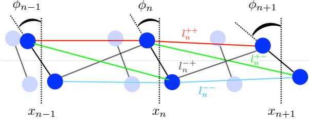
FIG. 5. (Color online) The diagram introduces the notations used in the text. The array of dimers is shown at the equilibrium (faded) and at some arbitrary snapshot in time.  $x_n$  represents the position of the center of mass of the  $n$ -th dimer and  $\phi_n$  represents the angle of rotation of the  $n$ -th dimer relative to the vertical axis. In the equilibrium configuration, all  $\phi_n$  are equal to  $\phi_0$ .
