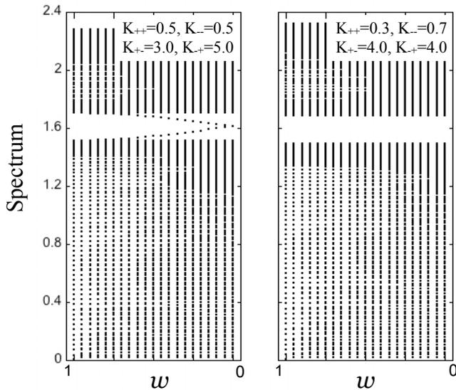
FIG. 8. Each vertical sequence of dots represent the frequencies of the normal modes of a chain made of 100 dimers arranged in a circle. The spring constants  $K$  of the springs connecting two dimers were gradually weakened by making the substitution  $K \rightarrow wK$  and letting  $w$  vary from 1 to 0. The frequencies were recomputed for many  $w$  values. Panel (a) refers to the topological case, and panel (b) to the non-topological case.
