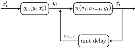
FIG. 9: An alternative representation to Fig. 1, where the strategy  $\pi(\sigma_t|\sigma_{t-1}, y_t)$  is viewed as a controller. The controller receives both feedforward information  $y_t$  through the sensor  $q_{\text{in}}(y_t|x'_t)$ , and feedback information  $\sigma_{t-1}$ , subject to delay (see also Table I).
