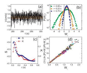
FIG. 3: (a) Typical velocity time series of polar particle without bead medium, at  $\Gamma = 3.0$ ; dashed line again indicates mean velocity. (b) Probability distribution of  $W_{\tau}$  for  $\tau =$ 0.06s, 0.22s and 0.70 s. (c) kurtosis (K) and skewness (S) as a function of  $\tau$  indicating tendency to become more Gaussian at higher  $\tau$ . (d)  $(1/\tau) \ln P(+W_{\tau})/P(-W_{\tau})$  vs.  $W_{\tau}$ , shows a collapse only for  $\tau \geq 0.20s$ .
