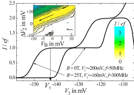
FIG. 2. (color online) Normalized current  $I/ef$  generated by electrons emitted into drain as function of  $V_2$ . The quantized regime  $I = ef$  under  $B = 0$  and  $B = 25$  T conditions is obtained over a  $V_2$  range of several mV. The threshold voltage  $V_T$  is indicated by the dashed arrow, beyond which the quantized regime breaks down. Inset showing  $I/ef$  as the bias  $V_B$  is varied.
