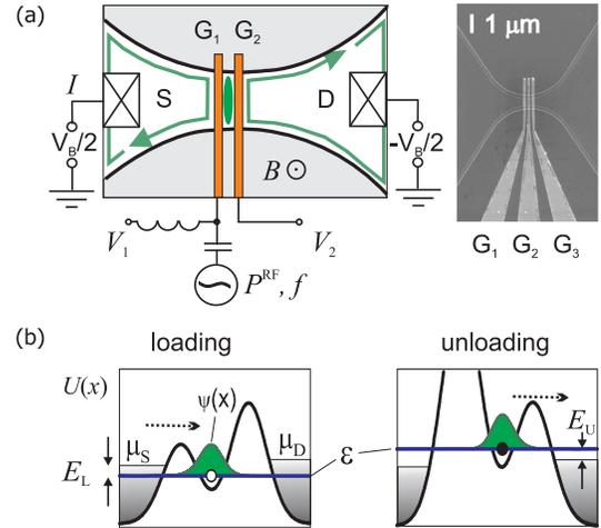
FIG. 1. (color online) Description of the device and operating principle. (a) Left, schematic of the device. Electron micrograph of the sample shown on the right. (b) Schematic of the potential energy landscape along the channel for the stages of loading and unloading.
