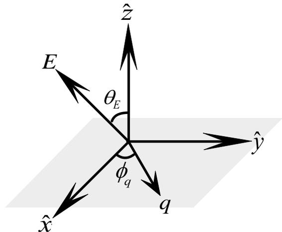
FIG. 1: (Color online). Schematic sketch of the 2D monolayer dipolar system in momentum space. The polarization direction of dipolar molecules is controlled by the external electric field  $\vec{E}$ , which is in the  $xz$  plane.
