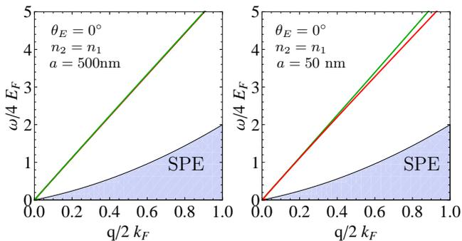
FIG. 3: (Color online). Calculated plasmon mode dispersions of bilayer dipolar system for two different interlayer distances (a)  $a = 0.5\mu\text{m}$  and (b)  $a = 50\text{ nm}$  at  $\theta_E = 0^\circ$ . We use  $n_1 = n_2 = 10^8\text{ cm}^{-2}$  and  $r = 4.4$  and  $s = 31$  in this calculation. The shadowed region indicate the single-particle excitation (SPE) region.
