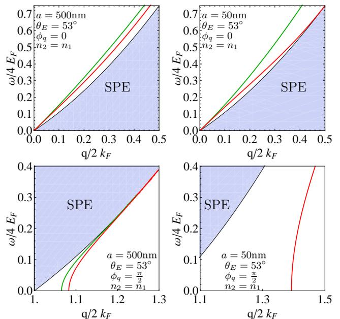
FIG. 4: (Color online). Calculated plasmon mode dispersions of double layer dipolar system for two different interlayer distance and  $\phi_q$  at  $\theta_E = 53^\circ$  with  $n_1 = n_2 = 10^8\text{ cm}^{-2}$ . The shadowed region indicate the single-particle excitation (SPE) region. The solid lines are solutions for  $\epsilon(q, \omega) = 0$  for  $r = 4.4$  and  $s = 31$ .
