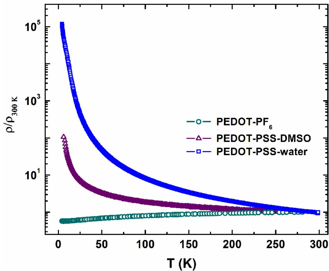
Fig.6. Temperature dependence of normalized resistivity of PEDOT-PSS in water and in DMSO solution, also compared with  $PF_6^-$  doped PEDOT.
