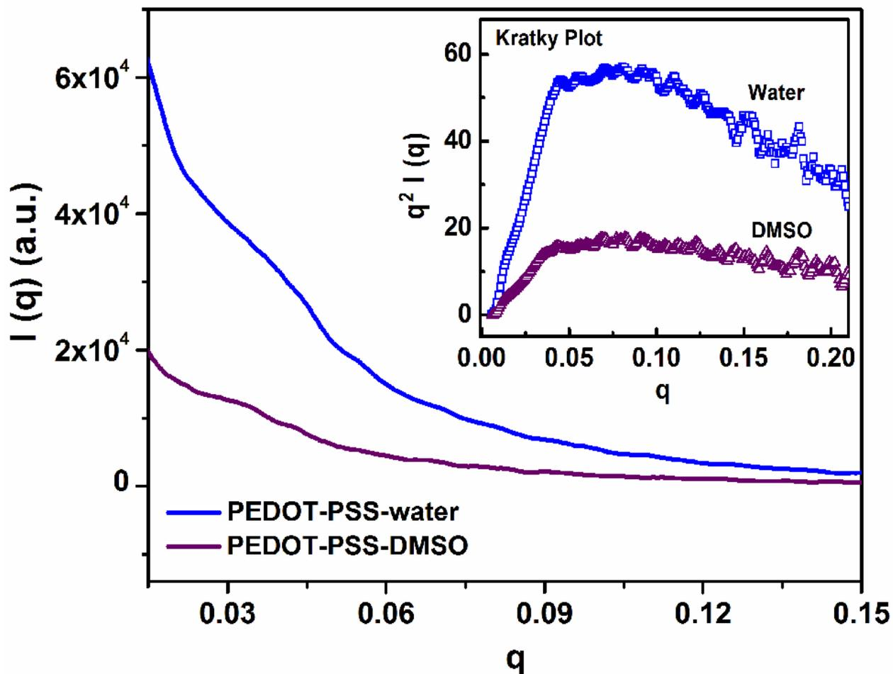
Fig. 3. Scattered intensity as a function of  $q$  for PEDOT-PSS solution in water and DMSO. Inset shows the corresponding Kratky plots [ $q^2 I(q)$  vs.  $q$ ]. A short plateau, with a rapid downturn from  $q = 0.1$  for aqueous solution implies compact coils. The broad plateau, with a weak downturn at  $q = 0.14$  for DMSO solution indicates extended coils, with more ordered features.
