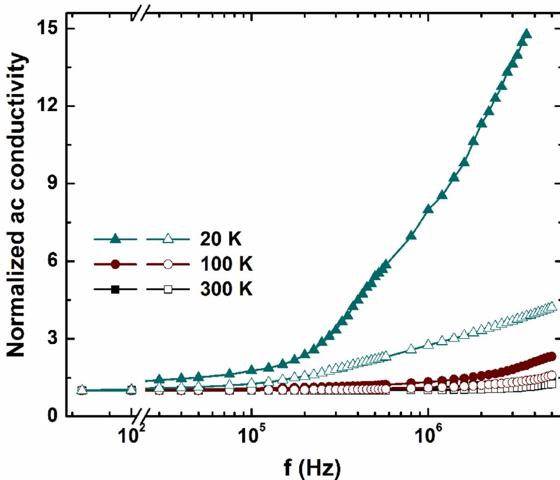
Fig. 7. Normalized ac conductivity of PEDOT-PSS in water (closed symbols) and DMSO (open symbols) at various temperatures.
