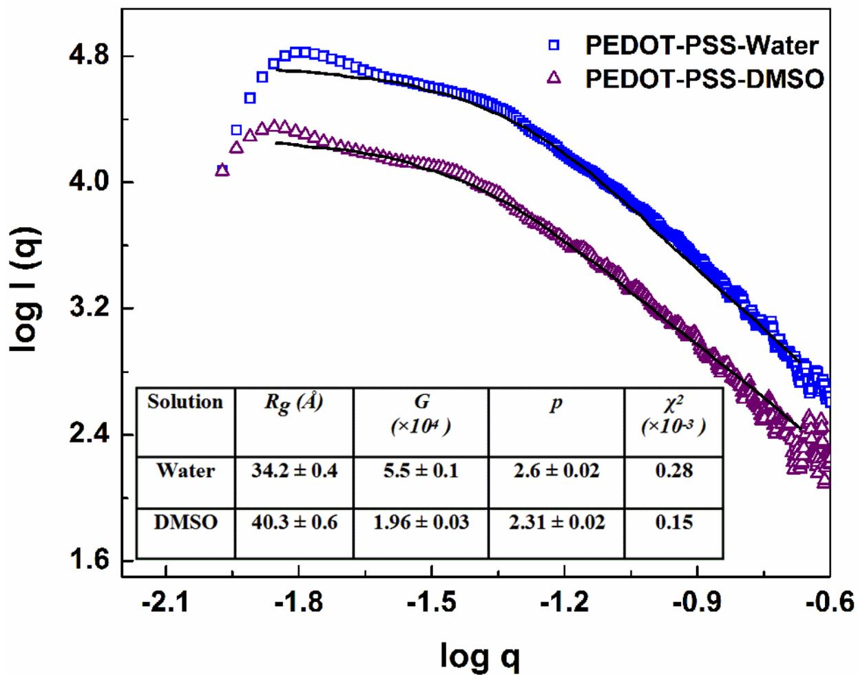
Fig. 4. Log-log plot of the scattered intensity as a function of  $q$  for PEDOT-PSS in water and DMSO solutions, and the linear region emphasizes power law behaviour. The solid lines are fits to Beaucage unified equation (Eq. 5). Inset-table shows the fit parameters.
