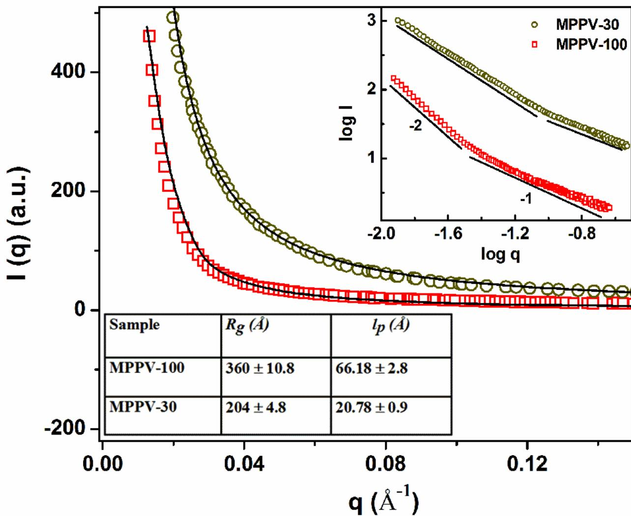
Fig. 2. Scattered intensity ( $I$ ) vs.  $q$  for M-PPV100 and M-PPV30 solution in xylene. Solid lines are fits to worm-like chain (WLC) model (Eq. 1). Inset-table shows the fit parameters. Inset-figure shows the corresponding  $\log I$  vs.  $\log q$  plots of the scattering profile.
