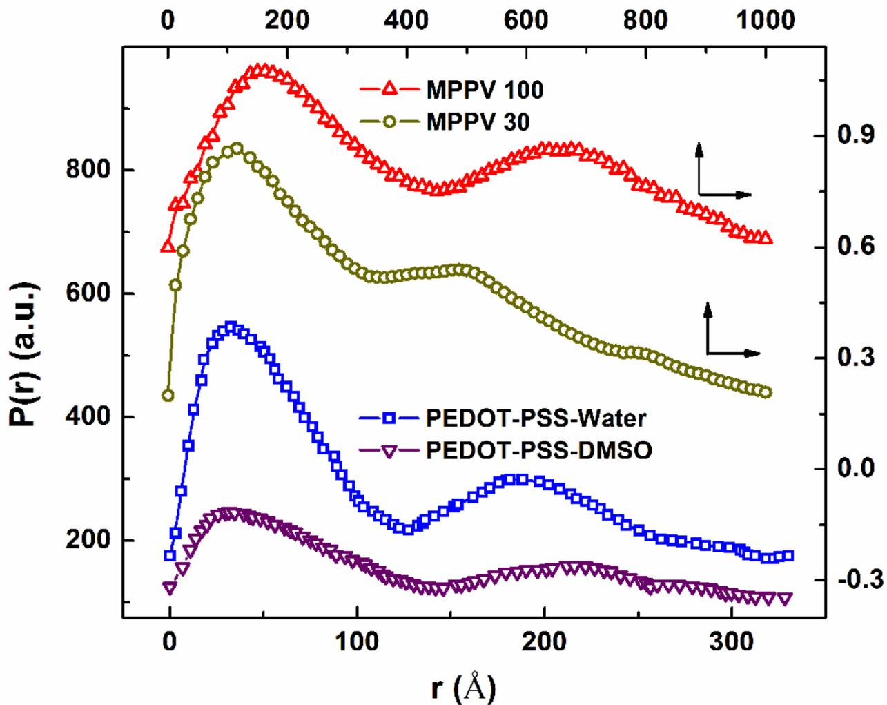
Fig. 5. Pair Distribution Function as a function of distance between scatterers ( $r$ ). PDF for both MEH-PPV and PEDOT-PSS are compared, as indicated by the arrows to the axes. The baselines are shifted for clarity. The first and second peaks show the correlation among intra & inter-chain segments respectively.
