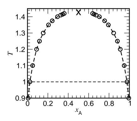
FIG. 1: Phase diagram of the symmetric binary (A,B) Lennard-Jones mixture, cf. Eqs. (7)-(10), in the plane of variables T and relative concentration of A particles ( $x_A = N_A/N$ ;  $N = N_A + N_B$ ) for fixed N = 6400. The cross shows the critical point, as obtained previously [47]. The horizontal broken line means that phase coexistence is studied at T = 1.0.
