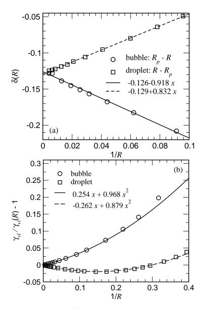
FIG. 17: (a) Radius-dependent Tolman length  $\delta(R) = R - R_p$  for bubbles and droplets with a corresponding linear fit in the range  $1/R \in (0, 0.1)$ . (b) Surface tension ratio  $\gamma_{vl}/\gamma_{vl}(R) - 1$  as function of the equimolar radius R for bubbles and droplets with a corresponding quadratic fit in the range  $1/R \in (0, 0.1)$ . All results are for the temperature  $T = 0.78T_c$ .
