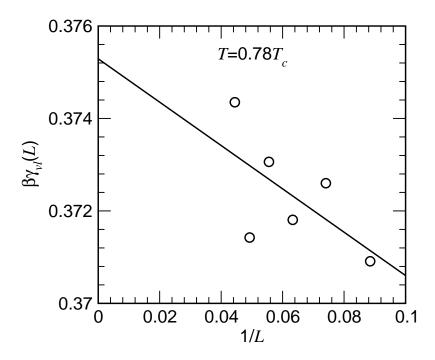
FIG. 12: Extrapolation of  $\beta \gamma_{vl}(L)$  as a function of 1/L for the simple LJ fluid at  $T = 0.78T_c$ , giving  $\beta \gamma_{vl} = \beta \gamma_{vl}(\infty) \simeq 0.375$ . Similar exercise at  $T = 0.68T_c$  gives  $\beta \gamma_{vl} \simeq 0.685$ .
