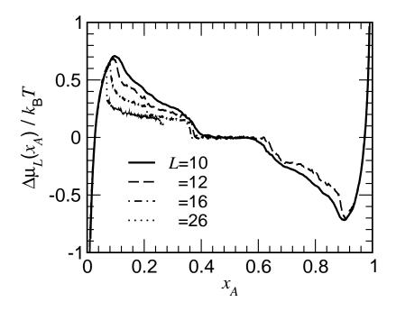
FIG. 6: Plot of  $\Delta \mu(X_A)/k_BT$  vs.  $X_A$  at T = 1.0 for L = 10, 12, 16, 26. Data refer to a single run at each size, to illustrate the typical noise level (200 Monte Carlo steps per particles have been used for each window of the successive umbrella sampling). For the final analysis, 5 such runs were averaged over.
