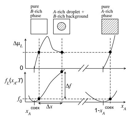
FIG. 7: Schematic explanation of how the estimation of the functions  $\Delta \mu_L(x_A, T)$  and  $f_L(x_A, T)$  together allows the estimation of the concentration difference  $\Delta x$  and free energy difference  $\Delta f$  due to a droplet.
