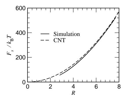
FIG. 8: Plot of  $F_S/k_BT$  of spherical A-rich droplet at T = 1 for the binary symmetric LJ mixture of Fig. 1. The description in terms of the capillarity approximation of classical nucleation theory (CNT) is shown as a broken curve, using  $\gamma_{AB}(\infty) = 0.722$  as obtained in Fig. 3. The full curve is a superposition of independent simulation results for L = 12, 16,18,20,22 and 24, where a running averaging was done using the combined data set.
