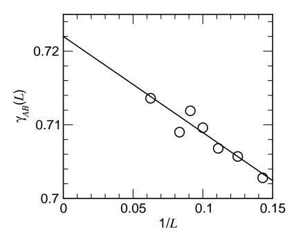
FIG. 3: Extrapolation of  $\gamma_{AB}(L)$  as function of 1/L, cf. Eq. (12), in order to estimate  $\gamma_{AB}(\infty)$ .
