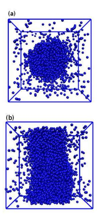
FIG. 5: a) Snapshot of a spherical droplet configuration formed by A particles in the background of B-particles (not shown), for T = 1.0, L = 24, and  $x_A = 0.15$ . b) Same as (a), but for a cylindrical droplet, choosing  $x_A = 0.27$ . Note that our method does not at all suppress statistical fluctuations in the size and shape of these droplets, which therefore have spherical or cylindrical symmetry on the average only.
