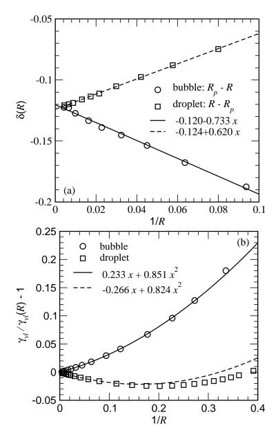
FIG. 18: (a) Radius-dependent Tolman length  $\delta(R) = R - R_p$  for bubbles and droplets with a corresponding linear fit in the range  $1/R \in (0, 0.1)$ . (b) Surface tension ratio  $\gamma_{vl}/\gamma_{vl}(R) - 1$  as function of the equimolar radius R for bubbles and droplets with a corresponding quadratic fit in the range  $1/R \in (0, 0.1)$ . All results are for the temperature  $T = 0.68T_c$ .
