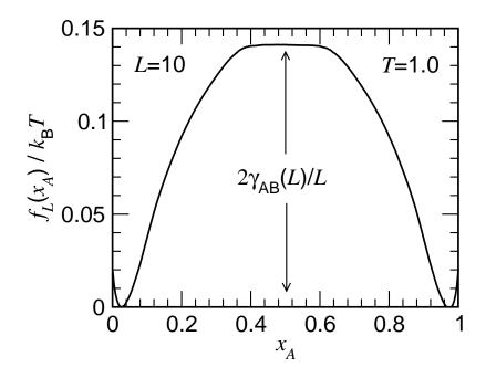
FIG. 2: Effective free energy  $f_L(x_A, T)$  of finite-size boxes of linear dimension L with L = 10 plotted vs.  $x_A$  at T = 1.0, for the model of Fig. 1. The estimation of the size-dependent interfacial tension  $\gamma_{AB}(L)$  is indicated.
