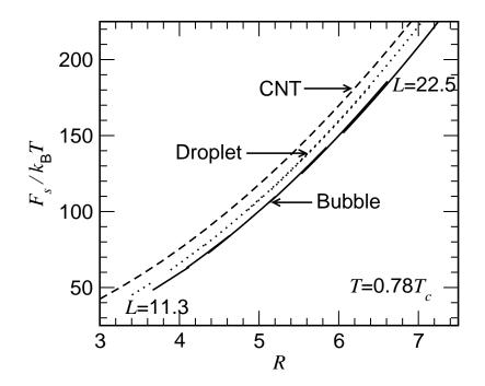
FIG. 13: Plots of  $F_S/k_BT$  of spherical droplets and bubbles for the one-component LJ fluid, at  $T = 0.78T_c$ , as a function of sphere radius R. The capillarity approximation (CNT),  $F_S/k_BT = 4\pi R^2 \gamma_{vl}(\infty)$  is included, using the estimate of  $\gamma(\infty)$  from Fig. 12.
