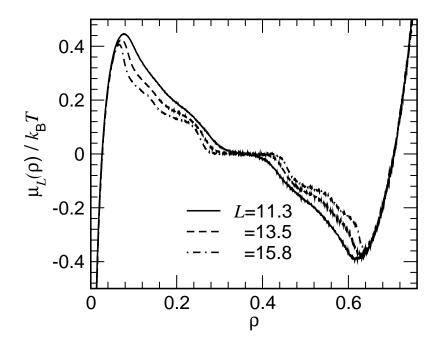
FIG. 11: Plot of  $\mu_L(\rho)/k_BT$  for the one-component Lennard-Jones fluid as a function of  $\rho$ , at  $T = 0.78T_c$ , for 3 values of L, as indicated.
