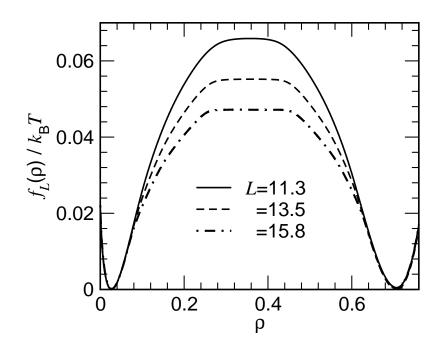
FIG. 10: Effective free energy density  $f_L(\rho)/k_BT$  of the single-component Lennard-Jones fluid at  $T = 0.78T_c$  plotted vs. density  $\rho$  for 3 values of L, as indicated in the figure.
