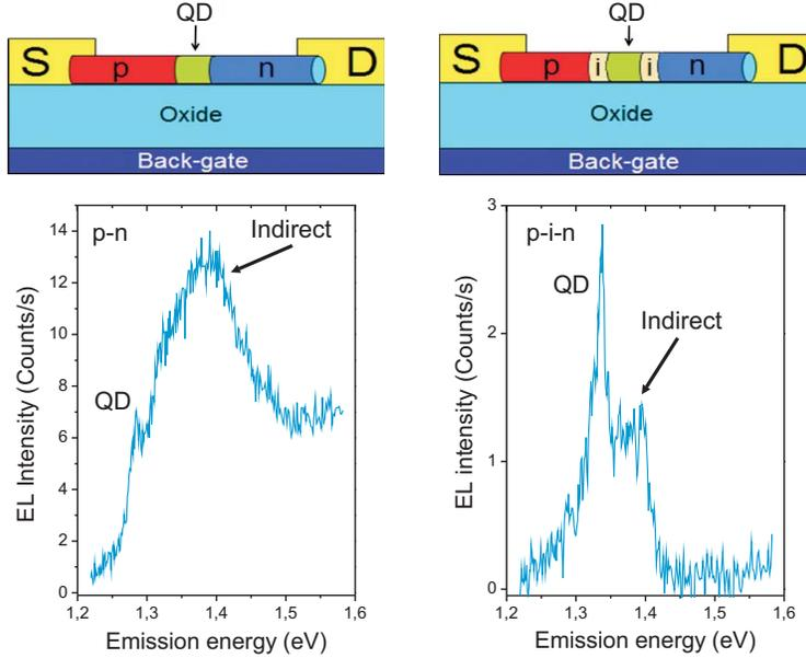
Figure 4. Comparison of low temperature (10 K) EL emission for p-n (left panel) and p-i-n (right panel) with an embedded InAsP quantum dot within the depletion region. The injected current for both EL spectra is  $\sim 100$  nA. The broad emission peak (indirect transitions) are suppressed in the p-i-n structure as compared to the p-n structure. A schematic view of the p-n and p-i-n structures is shown in the upper panel. S, source for the p-contact; D, drain for the n-contact.
