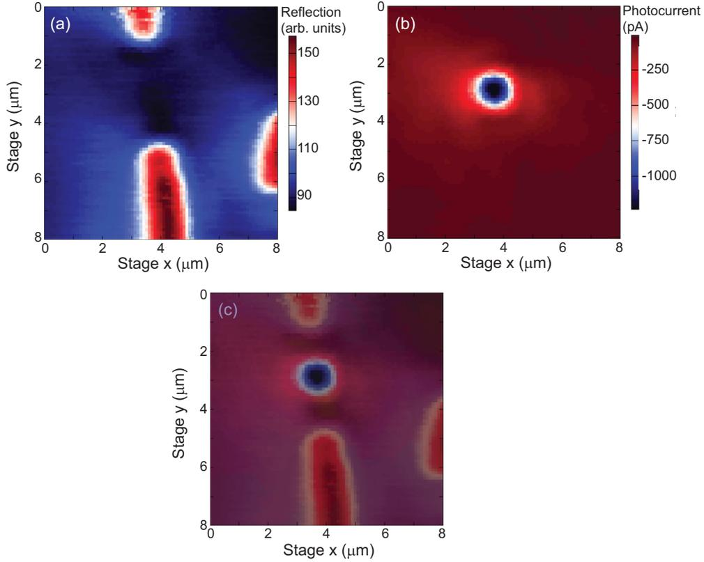
Figure 7. (a) Reflection image and (b) photocurrent image, which are both simultaneously acquired as a function of laser position at low temperature ( $T = 20$  K). (c) The reflection and photocurrent images from (a) and (b) are superimposed on the same image. We conclude from this image that the photocurrent, and thus multiplication, originate from within the depletion region (intrinsic section) of the Si nanowire.
