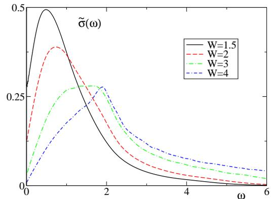
Figure 1. (Color online) Dynamical high- $T$  conductivity  $\tilde{\sigma}(\omega)$  for  $\Delta = 0.5$  and different disorders  $W = 1.5, 2, 3, 4$  evaluated for a half-filled system  $n = 1/2$  and  $L = 24$  sites.
