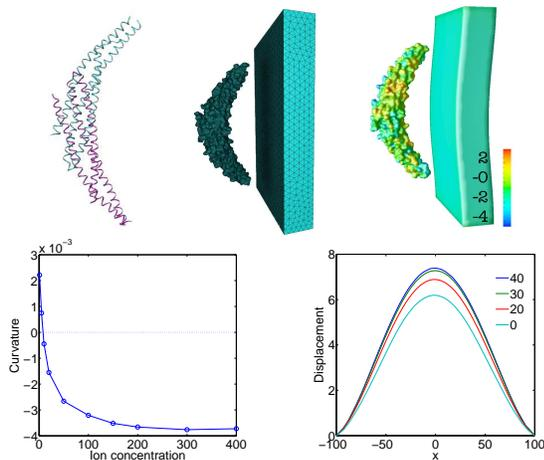
FIG. 3. First row: The structure of protein II4D (Left); Surface triangulation of the BAR-domain protein-membrane complex (Middle) and the electrostatic potential on the protein and membrane surfaces (Right). Second row: Membrane curvature at various ion concentrations (Left) and membrane displacement at various initial separations  $D$  (Right).
