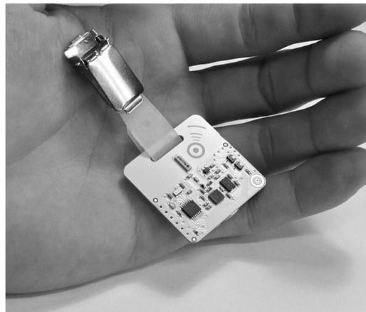
**Figure S7.** Active RFID tag used in the experiments. The RFID tag is based on an open design by the OpenBeacon project and features a microcontroller, a radio transceiver operating in the 2.4 GHz ISM band, an antenna embedded in the printed circuit board, and a lithium battery.
