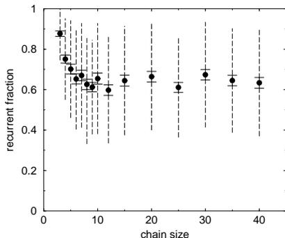
Fig. 3: Ensemble-averaged fractions of trajectories  $T$ -recurrent at  $T = 2 \cdot 10^5$  versus chain size, for random single-site initial conditions with  $0 < \mathcal{N} \leq 20$  and disorder strength  $W = 12$ . 100 different realizations were used for each size, and dashed lines show the standard deviations of the distributions. Trajectories were considered  $T$ -recurrent if  $\Lambda(T) < 10^{-4}$  (cf. fig. 2).
