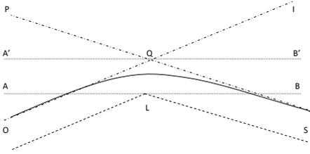
FIG. 2: Gravitational bending geometry when the source (S) and the observer (O) are at infinitely large distance away from the lens (L). AB is the polar axis,  $A'B'$  is parallel to the polar axis passing through the point Q, I is the image position, R is a reference object
