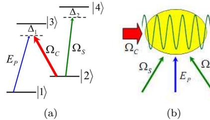
FIG. 1: (a) Energy diagram of the system. (b) Geometric configuration of the lights. Lattice-forming beams  $\Omega_S$  and nonclassical light beam  $\hat{E}_P$  are co-propagating, The coupling light  $\Omega_C$  is a p-wave, which is propagating transversely along the atoms
