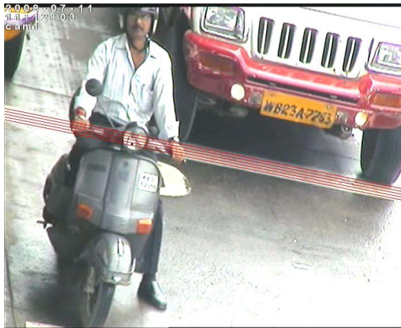
Fig. 4. A sample violating vehicle image with potential occlusions on the stop-line (hypothetically marked with a band of red lines).
