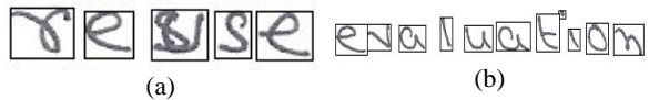
Fig. 7. Some of the misclassified word images (a) Recognition error in the 3 rd character (b) Internal segmentation in the 8 th character
