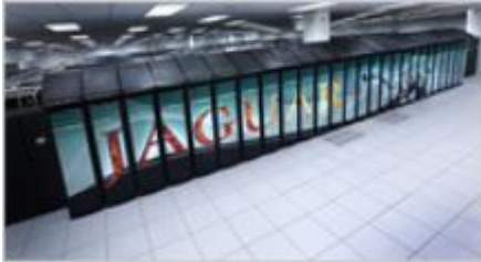
Fig.1 Jaguar supercomputer at the Oak Ridge National Laboratory, the world's fastest, links thousands of mainstream chips.
