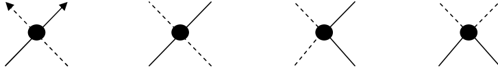
Figure 14: The three transitions at a vertex, in relation to an oriented Euler circuit: one transition follows the circuit, the second is consistent with the edge-directions determined by the Euler circuit, and the third is not consistent with these edge-directions.
